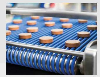
This machine, consisting of four aligners, is located between the extruder and the coating belt and optimises the productive capacity of the line. By making use of an oscillatory motion with adjustable steps the product is sorted into lines, transported towards the coating zone and subsequent cooling in the tunnel. It should be noted that the entire process is automated and does not require the manual input of the operator, hence avoiding damage to the previously extruded product.
