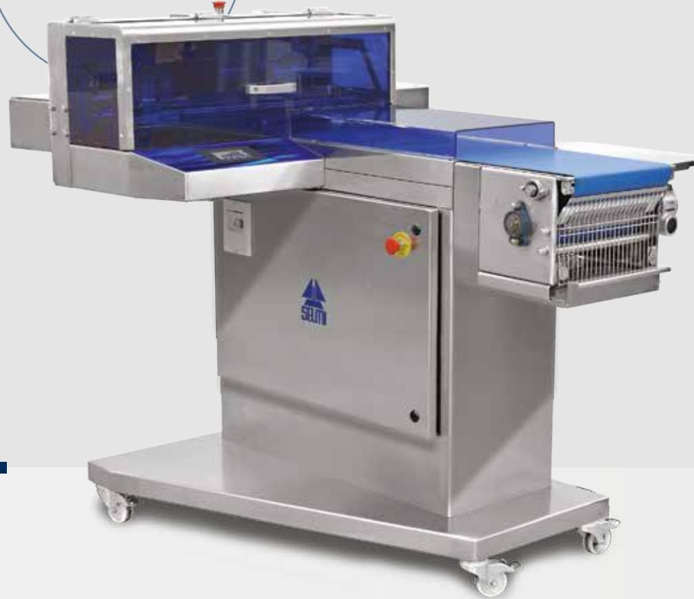
This machine is designed to carry out the automatic demoulding of pralines or bars that are held inside moulds
