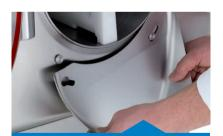
The extraction chute is removable to facilitate the removal of all gelato, cream, or chocolate residue, for complete cleaning.
