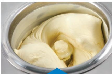
**Static Storage.** At the end of the batch freezing cycle, the Gelato is automatically stored inside the cylinder and ready to be served. There is no need to extract into another container and blast freeze it since there is no thermal shock. The ideal storage temperature for each flavor can be independently set and adjusted at any time.
