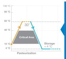
**Standard**. With the automatic **self-pasteurization** system you can choose when to wash the machine up to a maximum interval of 42 days. As a further guarantee of hygienic safety, if the operator does not perform the complete cleaning at the end of the set days, the machine goes into automatic block.
