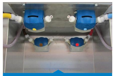
Automatic syrup dispensing system (only for K Shake). At the time of dispensing, the operator can therefore choose between 5 shake options: neutral, or variegated with one of the 4 syrups. Thanks to the peristaltic pumps that can manage up to 4 syrups at the same time.
