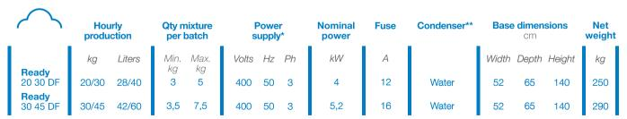
The quantity per batch varies depending on the mixtures used. The hourly production refers to the use of readymade mixtures. The maximum values refer to traditional Italian gelato.
