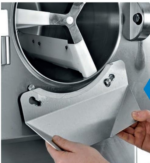
**The cylinder and front panel are a single piece** for maximum cleanliness and hygiene.
